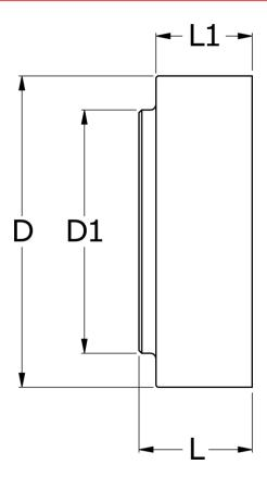
D = 110 D1 = 86 L = 40 L1 = 34 Max bore = 48 Torque (N m) = 160
